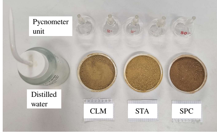
Figure 6: Pycnometer test soils and setup.
